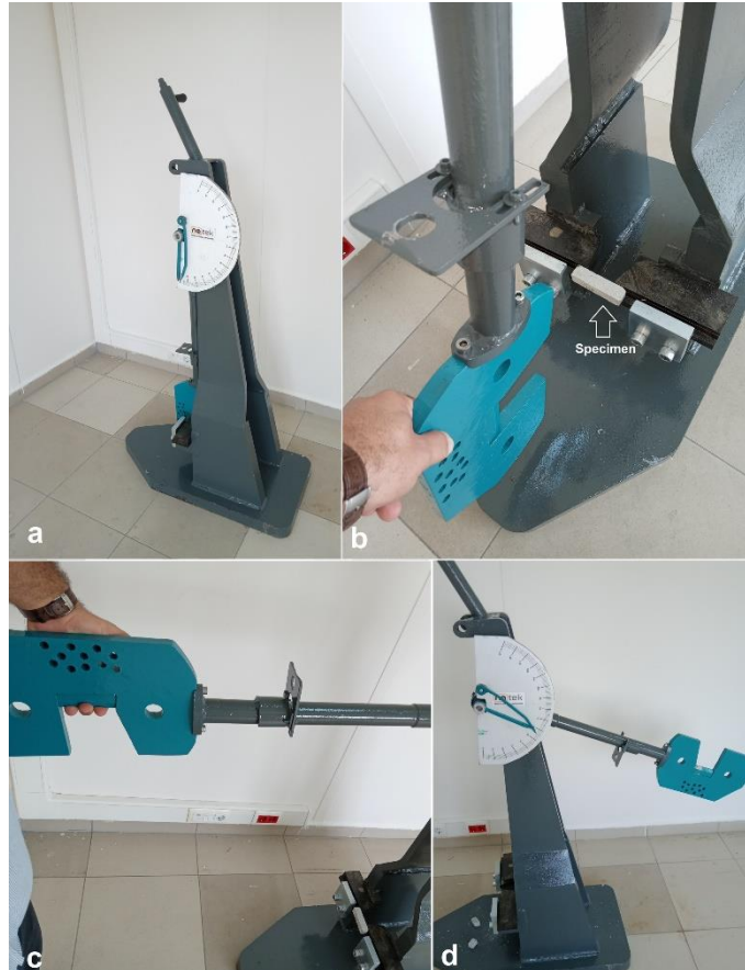
Figure 2. a) The Charpy impact test equipment, b and c) raising the hammer, d) hammer after fall
