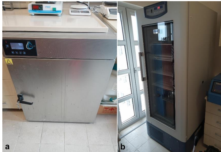
Figure 3. Stove (a) and refrigerator (b) used in the thermal cycles
