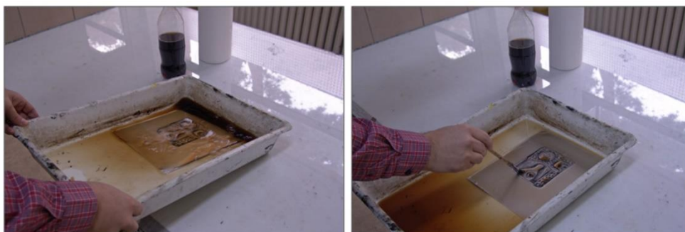
Figure 7. Corrosion of foil with cola
