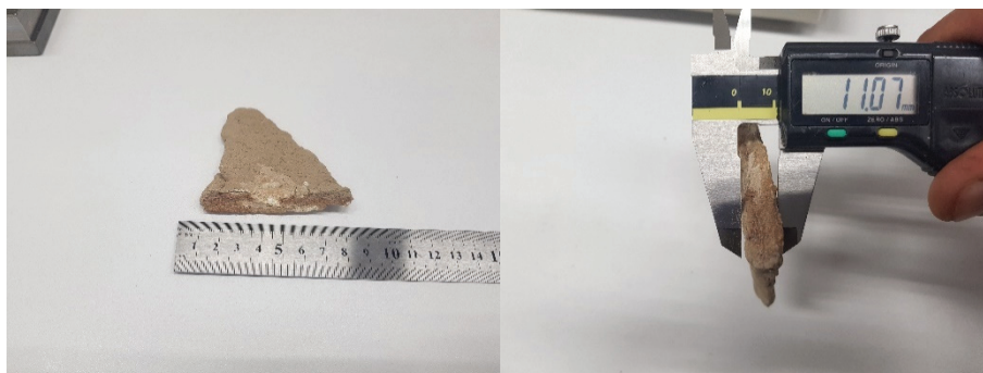
Figure 5 - Calcinated sample from penstock
