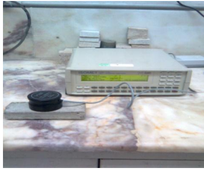
Fig 2.2. Isomet 2104 portable heat transfer analyzer
