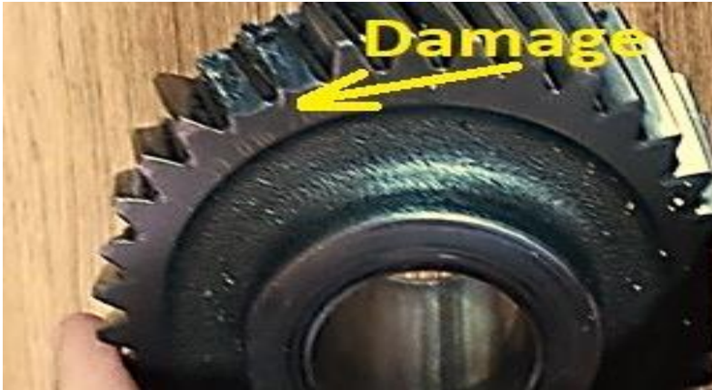
Figure 4. The damaged helical gear wheel.
