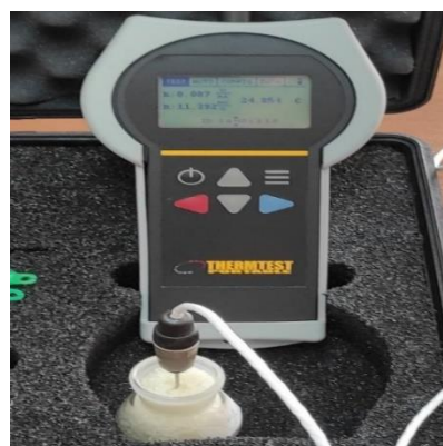
Figure 5. Thermal conductivity tests applied to aerogels.
