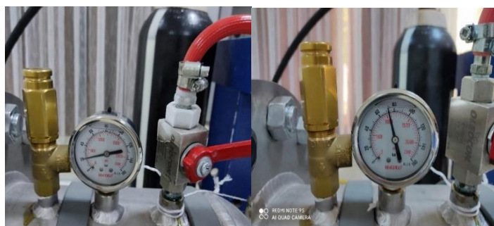
Figure 3. CO 2 reaching supercritical state in the reactor.
