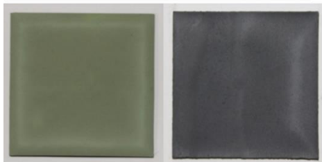
Cell 3 sintered with two 75x75 mm LxW porous alumina cover plates on the top of the cell, with a total mass of 32.9 g
