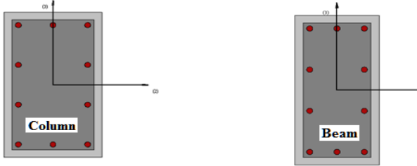
Figure 2. The cross-sections of columns and beams
