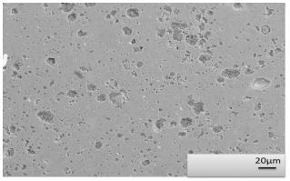
**Figure 5.** SEM micrograph of the tile surface coated with solution 4S at (80-90°C).
