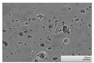
**Figure 8.** The microstructure of tile which was polished 10 cm distance between polishing heads.
