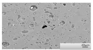
**Figure 4.** SEM micrograph of the tile surface coated with solution 4S at (60-70°C).
