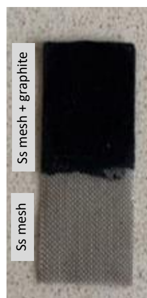
Figure 3. Stainless steel mesh + graphite electrode.
