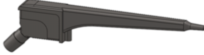
Fig. 1. Designed 3D model of the hip prosthesis
