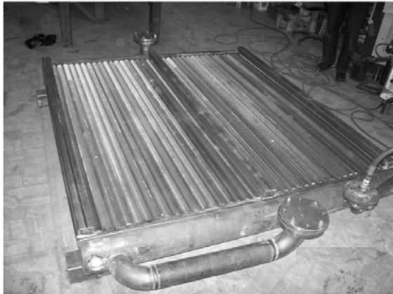
Figure 6. Pressure test of the heat exchanger
