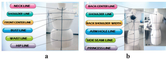
Figure 3. Line tape draping
