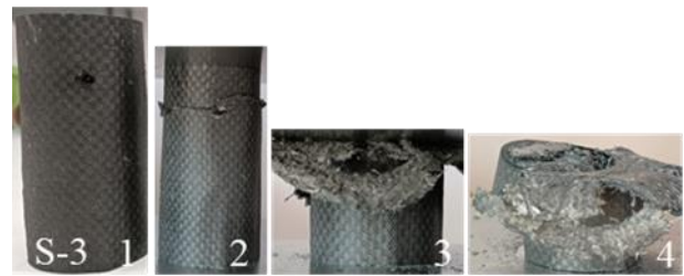
Figure 9. Damage of S-3 specimen during quasi-static compression
