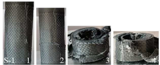
Figure 5. Damage of S-1 specimen during quasi-static compression
