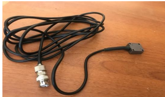
Figure 4. An example of the accelerometer sensor used
