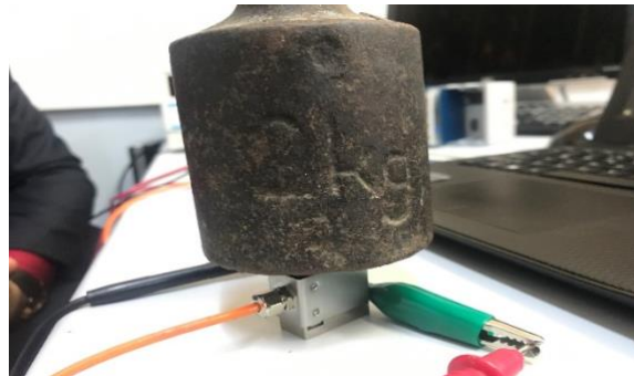
Figure 2. Test of the load cell
