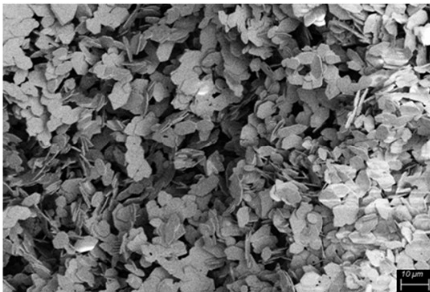
Figure 4. SEM image of copper hydroxynitrate.
