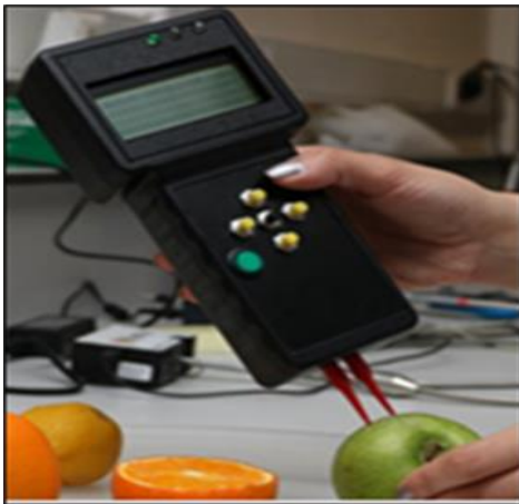
Figure 5. Freshness measurement of apples by using the first prototype
