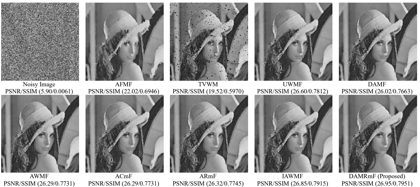
Figure 2. Image denoising results of the compared filters with SPN level of 90% of the "Lena" image (512 × 512 pixels).
